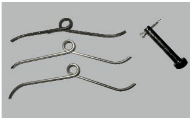
Photo 2: Springs and pivot pin. Springs from top to Bottom: Original spring; Replacement spring modified as described; Replacement spring as supplied.
