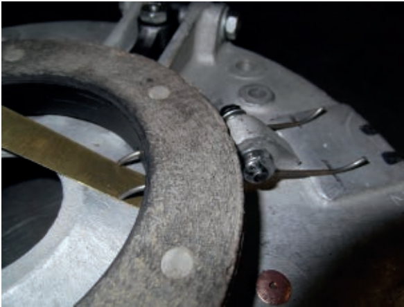
Photo 1: Clutch assembly with springs in place with a 10 thou feeler gauge under the spring end; this is a more than adequate gap.
