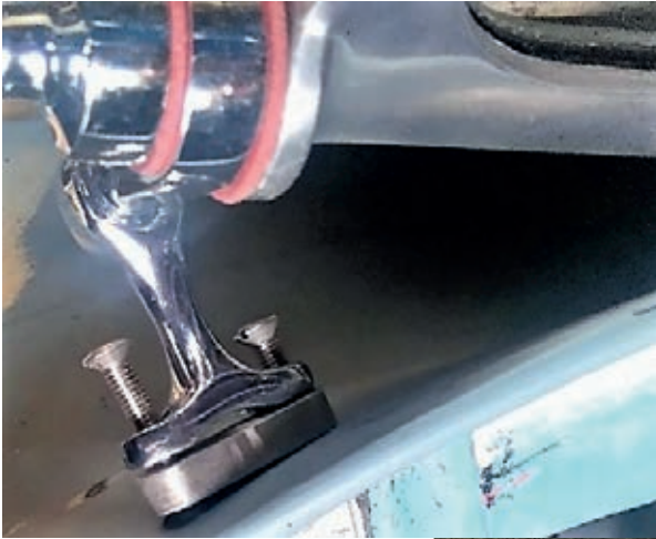
Stainless steel spacers in position
