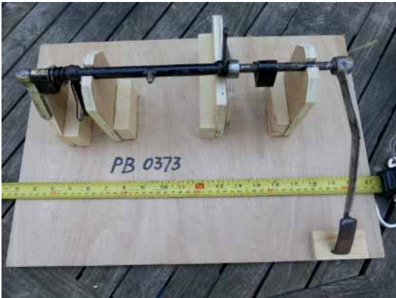
Old throttle shaft used to make the assembly jig
