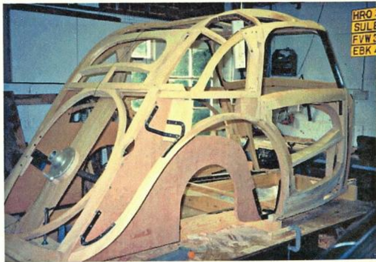
Geodesic timber - the complex frame under the Airliner coupe's smooth outer skin.
