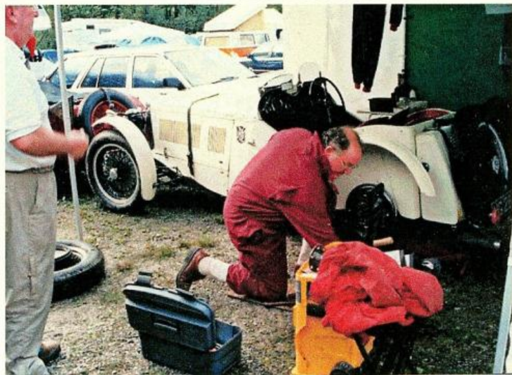
Bob Jones changing a halfshaft broken at Klausen Hill Climb Photo: B. Foster
