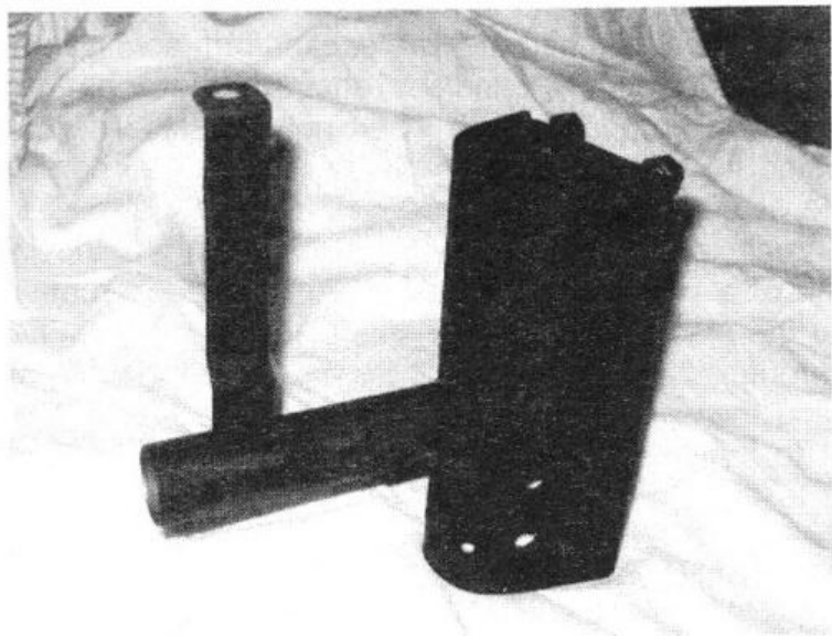
The exhaust heat collector box, with connector pipe to the air box
