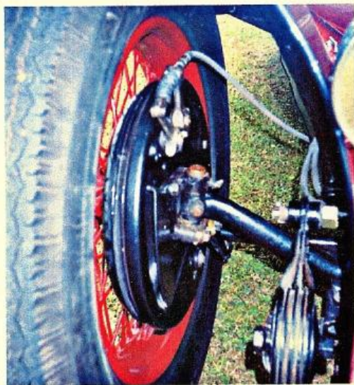
Twin lever brake conversion on Alan Hogg's ND
