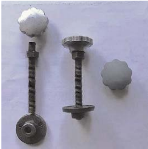
Original adjusters together with the 3D printed master pattern on the right (grey)
