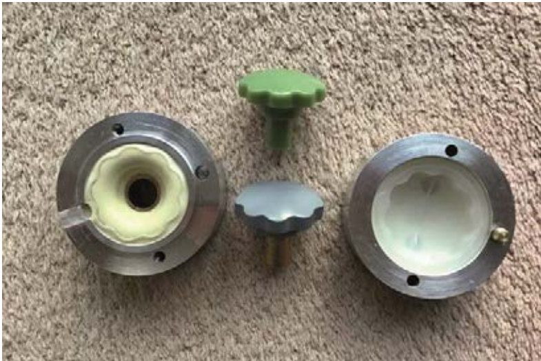
The two halves of the mould, the master pattern (grey), and the wax pattern produced by the mould (green)
