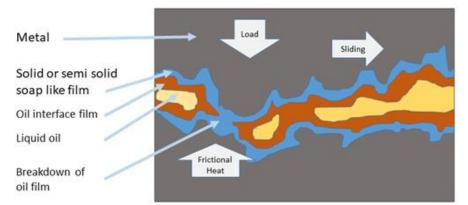
(AW) agents are polar additives that react with the metal when metal-to-metal contact occurs. Activated by the frictional heat, they form a wax like film that protects the metal surface. In the process, the levels of these additives in the oil drops.
