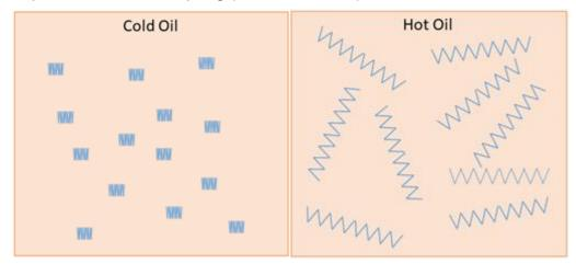
At low temperatures it is coiled up like a ball and has very little effect on the ability of the oil to flow. As the temperature increases, the spring expands, thickening the oil and reducing its ability to flow. This increases the natural viscosity of the oil at these higher temperatures.
